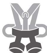
The sit harness is a textil element encircling the waist, connected to each leg and provided with a ventral attachment point allowing the suspension of a person.
