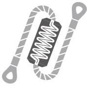
Energy absorber is obligatorily used in situation where the user is exposed to fall risks. The lanyard has to dissipate the Energy developed during a fall from a height and to reduce the braking force to a no lesional level.
