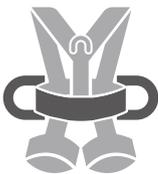
The work positioning lanyard links the belt to the anchoring point (restraint), or to a surrounding structure to allow to free the hands (work positioning). The work positioning lanyard connects a belt at an anchor point (restraint), or a structure surrounding it, so to be able to let go of the hands (maintenance at work). In this case, use with a fall arrest system.
